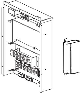
Step 2. Assemble the cover of independent power module, fix it tightly with bolts and connect wires.
