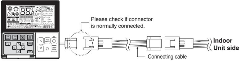
5. Please use extension cable if the distance between wired remote controller and indoor unit is more than 10m.
