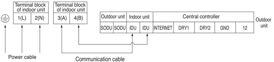
**WARNING :** Make sure that the screws of the terminal are free from looseness.
