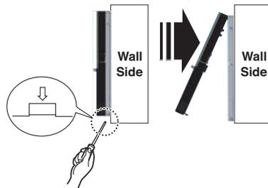
When separating remote controller from setup board, as the picture below, after inserting into the lower separating hole using screw driver and then, spinning clockwise, remote controller is separated.
