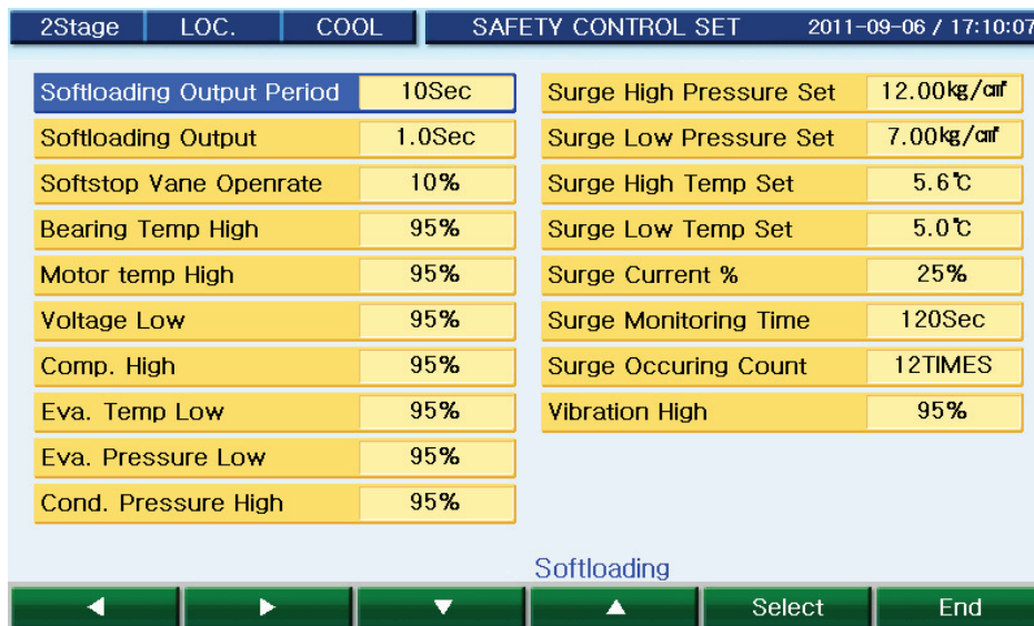
Fig 41. Safety control setting screen
